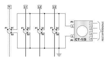
is the eventual separation of a transformer from the parallel, during low load demand periods. In this case the eventual clg is totally re-closed through the earth of an unique transformer and the tripping threshold should be establish exactly as 5A, under these conditions. The solution of the problem is given in our diagram.
