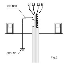
**NOTE** If there is an earthing circuit, it should be placed outside of the T/T (fig1). When the cable is fitted with a metallic screen and it gets through the T/T, the earthing connection should be as (fig. 2).
