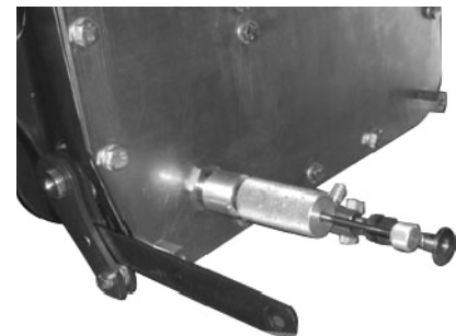
Connect the vacuum/filling device.
