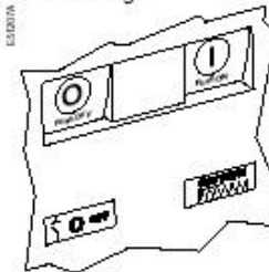
Circuit breaker open and discharged
