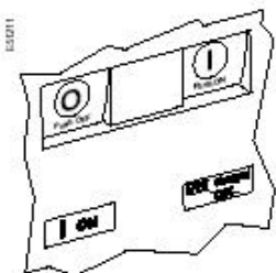
Circuit breaker closed, charged and not "ready to close"
