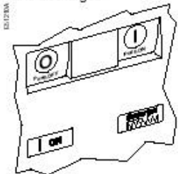
Circuit breaker closed and discharged
